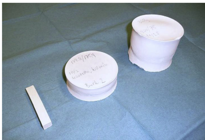
Fig. 4. Three examples of compacts made by hydration under pressure of 10, 150 and 300 g of calcium sulfate hemihydrate and stoichiometric amounts of water (19 wt%).
